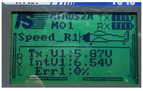
Handheld Transmitter (TX / TX.V1) Voltage 6.0+ volts to show full charge.
